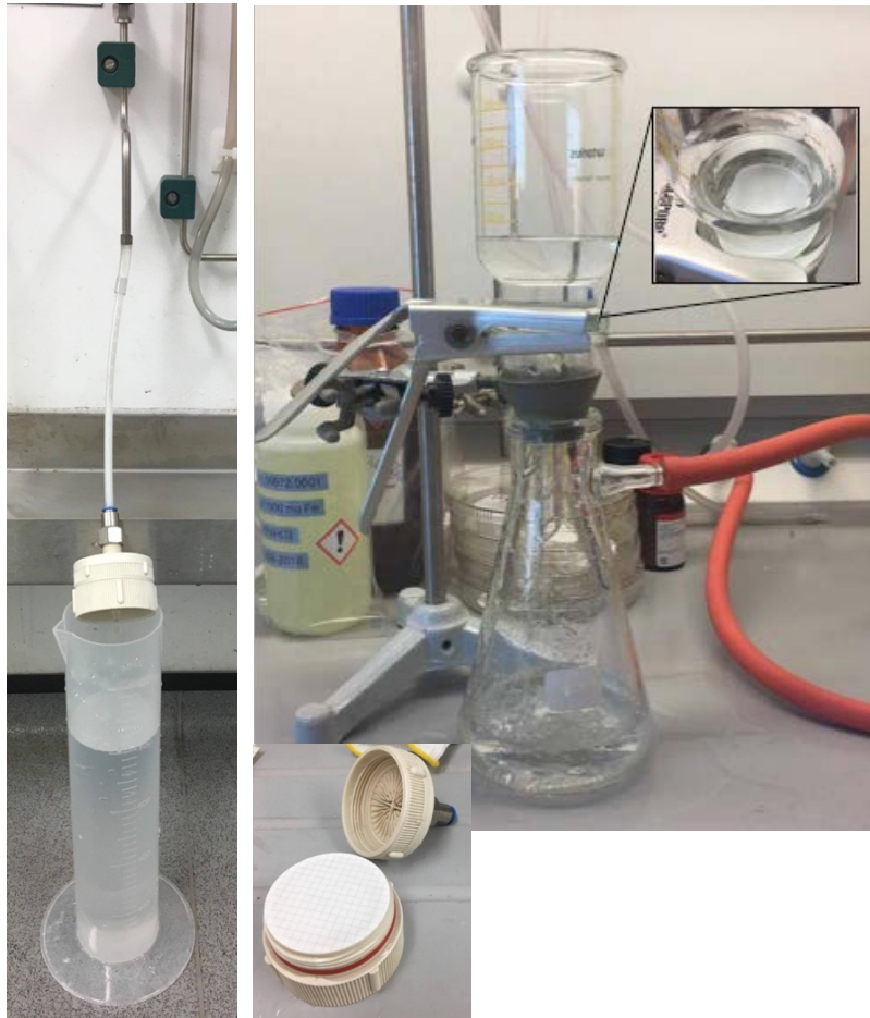
Figure 1. Filtration of filtered iron samples on-site or after sampling in the laboratory. The filter holder may be connected to the sample point by a flexible tube and a clamp.
